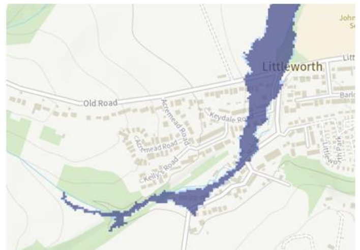
Figure 2: Flood Map for Littleworth showing the brook entering from the Northwest and running down along the cutting.
