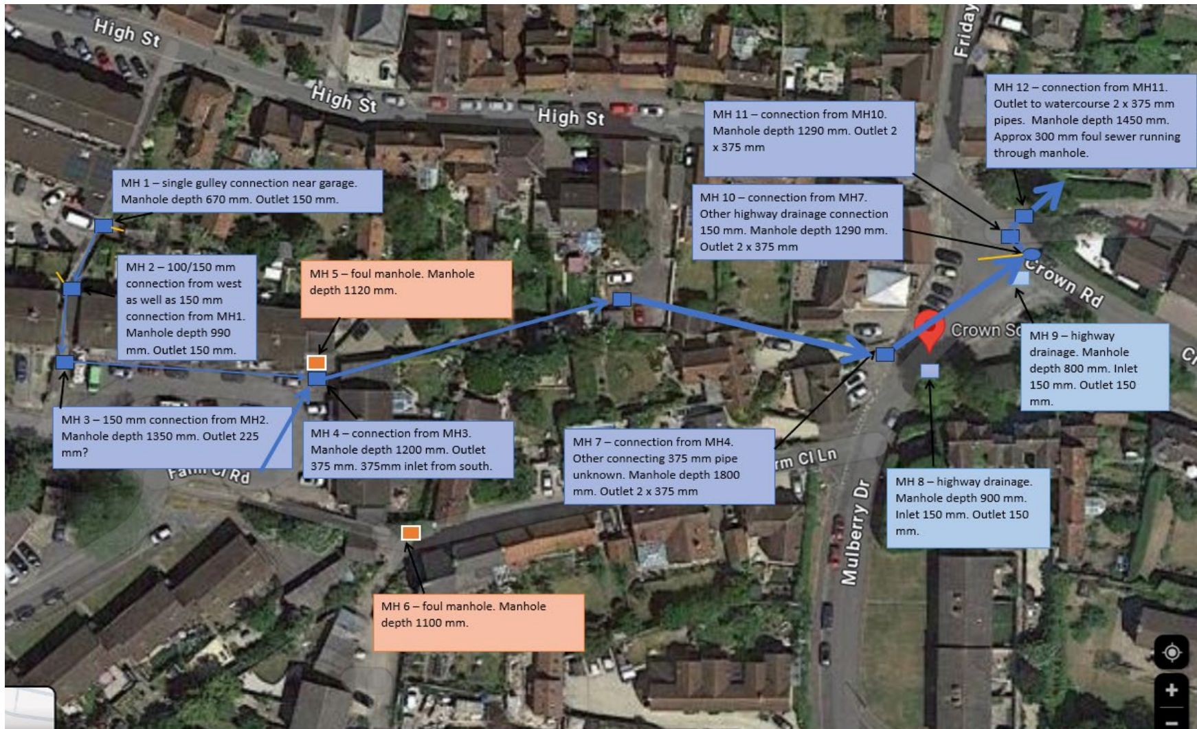
Figure 16 - Surface Water drainage network around Crown Square. (Contains Ordnance Survey data © Crown copyright and database right 2024 [1000018668].
